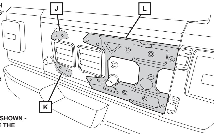
**SWING GATE REINFORCEMENT KIT (J)(K)(L) SHOWN - IS REQUIRED TO BE INSTALLED BEFORE THE INSTALLATION OF THIS KIT.**
